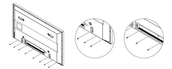
2 Set the Speaker Guide Bracket into the square grooves located on either side of the PDP's bottom rear, then push the Speaker Guide Bracket towards the center (as the arrow illustrates). Secure the Speaker Guide Bracket with provided screws (2). Secure the Middle Cabinet to the center of the PDP with a screw (1). (Always use the proper screws, as indicated.)
